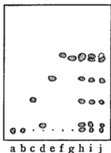
Fig. 4. Thin layer adsorption chromatographic separation of cholesterol, cholesterol ester and triglyceride involved in organic soils.
